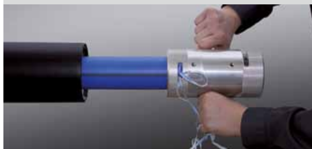
Pre-turn the peeling tool as far as it will go. The circumferential material abrasion is conveyed at one side of the tool.
