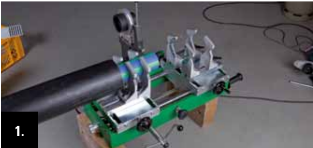
1. Position and align the welding machine. Regard the required place! (Consider that the machine must be removed below the pipeline after finishing the welding works.)
