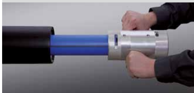
Push the aquatherm- peeling tool on the pipe end and turn it clockwise with pressure.
