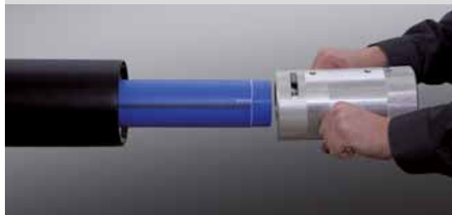
At the stop of the peeling tool the barrier layer is removed up to the welding depth. Now the tool can be pulled off.
