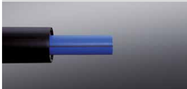
aquatherm blue pipe or ti is coated with an oxygen barrier, which must be removed before the fusion.
