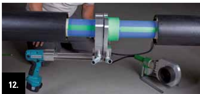
12. Align the welding connection with the welding jig and fix it shortly. The further processing is proceeded after the specified cooling time.
